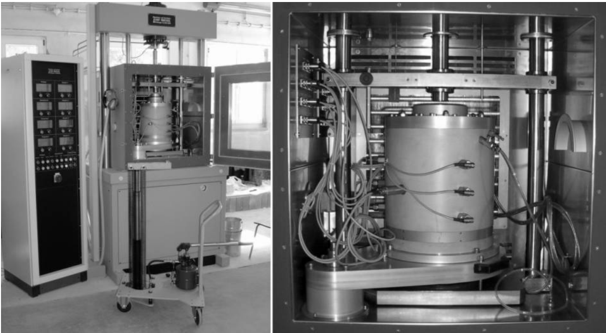
Figure 4: Universal Triaxial Testing Machine with climatic chamber
