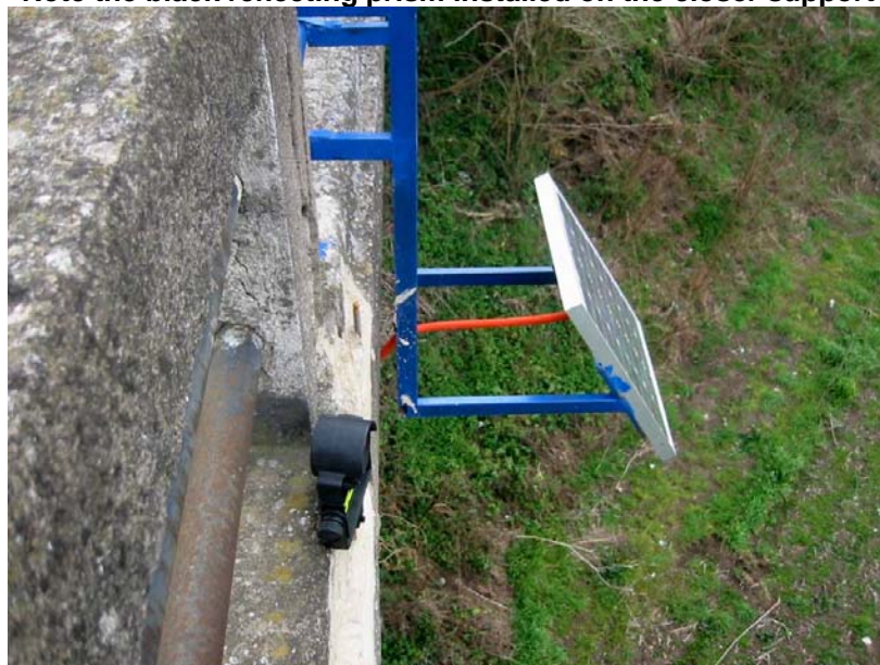
Picture 4: in this picture the solar panel and the topographic supports are visible. Note the black reflecting prism installed on the closer support
