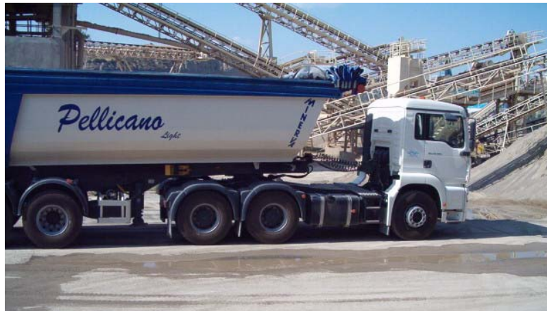
Fig.14: one of the heavy vehicle used to test the pavement
