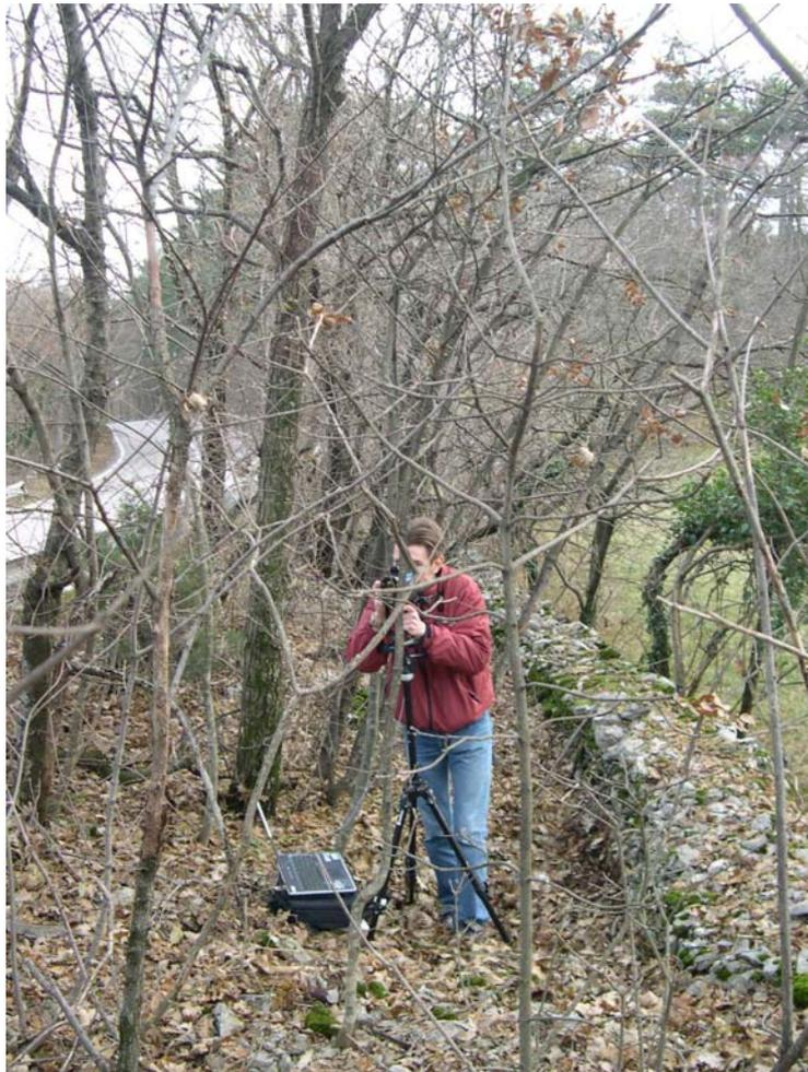
**Figure 1: Measurement hiding place with the Lidar gun on the tripod and the computer**
