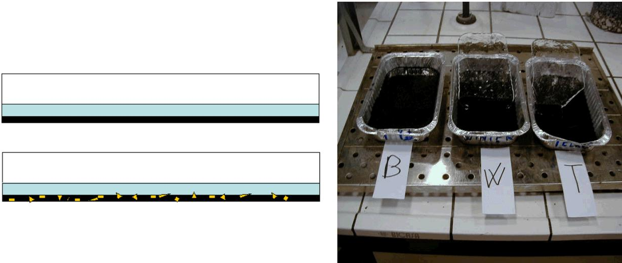
Figure 5 – Untreated bitumen film on the bottom of a container with a film of water and a film of bitumen previously mixed with anti-freezing products, also on the bottom of a container with a film of water, both to be placed in a freezer. In the photograph the new products W, with ordinary bitumen B and the first additive T.
