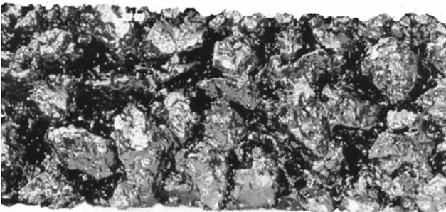
*Figure 1 – Cross-section of a draining pavement.
