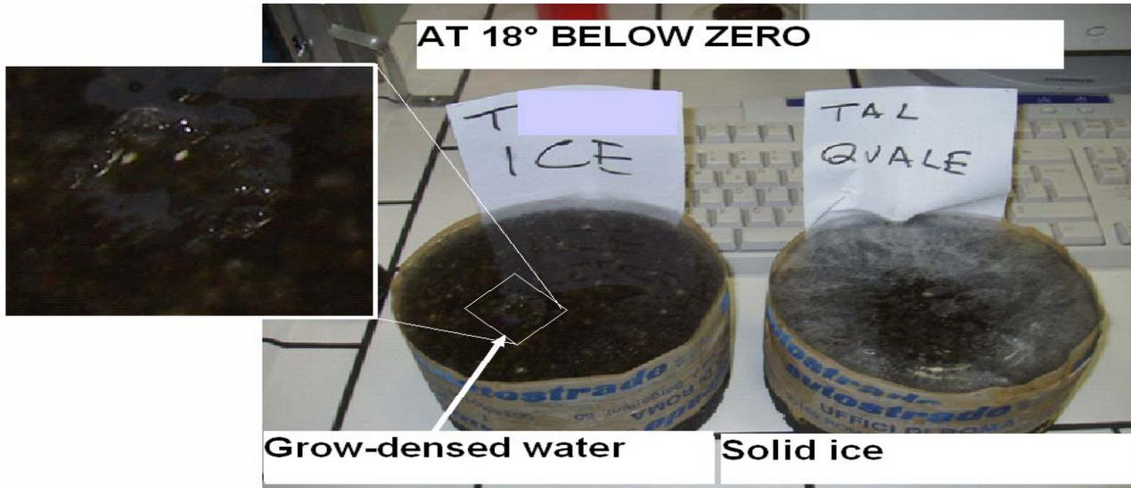
Figure 2 -Tests after freezing action 18° below zero. Note the type of ice found: only grow- densed water, with proactive fillers (left) ; solid ice, with pure bitumen (right)
