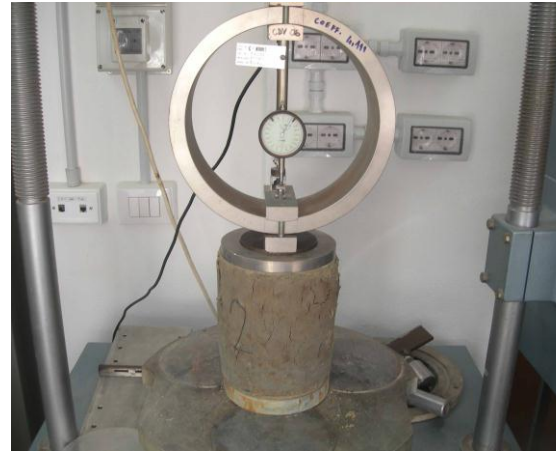
Figure 10 Specimen during compression strength test
