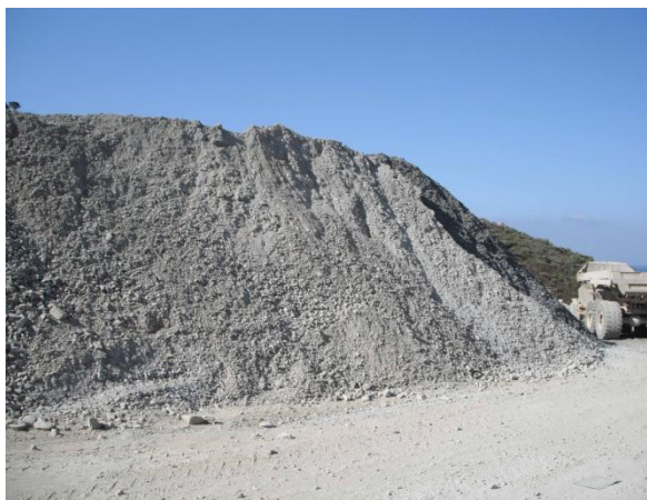
Figure 1- A Granite by-product deriving from TBM
